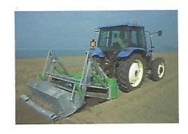
sand. The sand falls through the mesh while the waste is forced up the screen into a practical steel the waste basket which can be emptied hydraulically.
