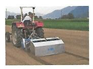
The Marlin B used a force fed system where a front blade is lowered into the sand by the operator within the tractor using the hydraulic lifter. The sand is forced onto a high frequency vibrating screen, which is then sifted to separate the waste materials from the sand. The sand falls through the mesh while the
